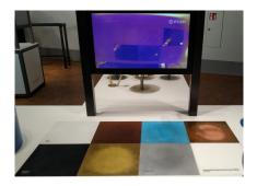
In the experiment, students try to understand the importance of thermal conductivity and how it changes according to the materials by touching objects made of different materials.
