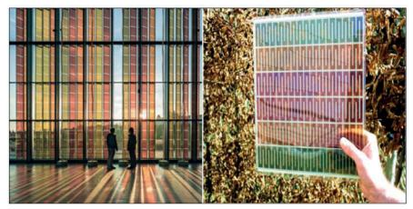
Micheal Gratzel developed solar panels that will enable electricity to be obtained from windows in homes and workplaces. This project brought him the Millennium Technology Award. Paint-sensitive solar panels, also known as Gratzel cells, are based on the principle of stimulating the dye between two glasses by light rays. This design is very similar to photosynthesis in living things. These panels are both transparent and cheaper than other Solar panels.
