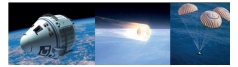
A space capsule is a simple-shaped spacecraft that can be used for reentry into the atmosphere without the use of wings or other features. As the space capsules return to Earth, their speeds reach 30,000 km/h, and their temperatures can reach over 1,500 degrees Celsius during their passage through the atmosphere. As a result, capsules require strong heat shields.
