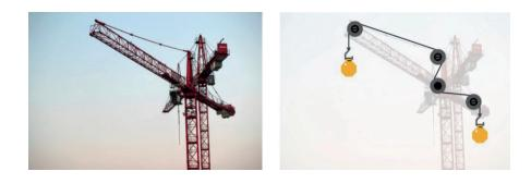
Tower cranes are essential for moving heavy goods, materials or tools around a site. They're great for speeding up construction, saving time and manpower. Tower cranes are impressive works of engineering. Their height can reach up to 75 metres and they can lift up to 20 tons.
